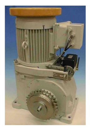
Picture 1: EC 2-15 Options: Weaterproof, Short Motor, Chain Wheel, Brake Function Sensors, Brake Lininig Wear Sensors
